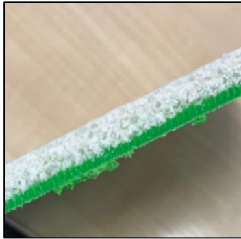
(Figure 5) PP (B) and Foam (A) blended on 50/50wt%.
