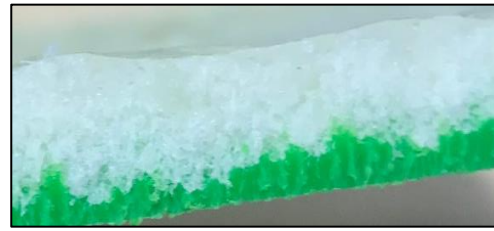
(Figure 7) PP (C) dry blended with Foam (A) 50/50wt%.
