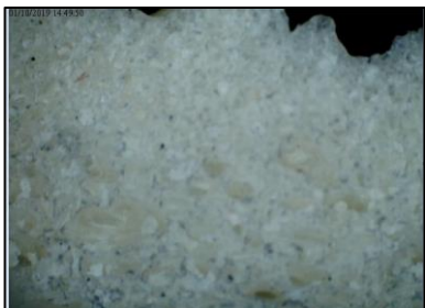
(Figure 12) 40 minute cell structure (40x optical zoom).
