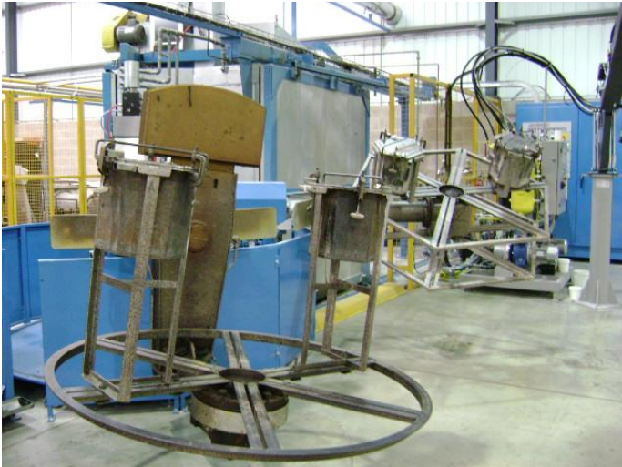
Fig. 2 – Test mould hex-bin on the Ferry RS 1.90
