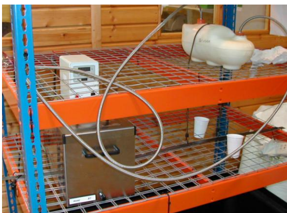
Figure 3 – System used to measure the operating temperature
