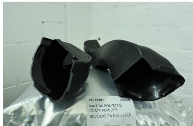
The mouldings have to withstand high temperatures, especially near the ceramic brakes, and they have to be tough, stiff and be light-weight and be made to very tight and exacting tolerances. Additionally the inner surface of the mouldings are fully visible at the front of the sports car, so they need to be as black and glossy as possible.
