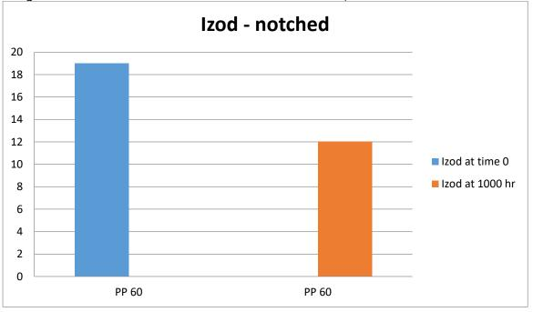
You can see that the material after 1,000 hours retained 63% of its original impact strength and easily passed the test.
