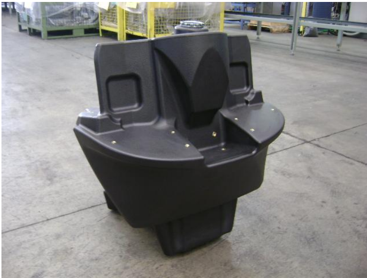
Diesel fuel tank for tractors
